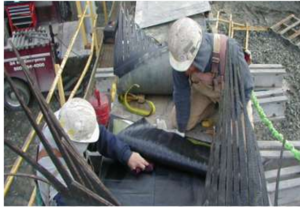
Conveyor belt joining (vulcanizing) and replacement (350 meters long) in ASK Gypsum, Yanbu,
